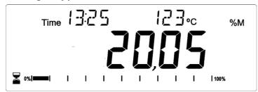
Showing a test in progress for 13:25, with a current temperature of 123°C and 20.05% moisture, the test is still running.
