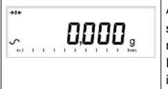
A stable sign ~ is shown when the PMB is in stable condition. It will turn off if the reading is not stable. Exact zero is shown when the "→0← " symbol is on to the left of the display area.
